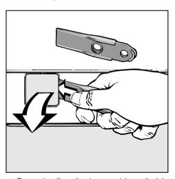
Open the flap (in the machine plinth).
